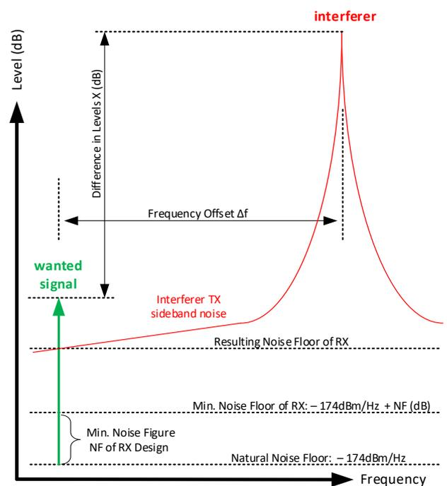
Δ Fig. 10 Key Parameters for collocated Installations
