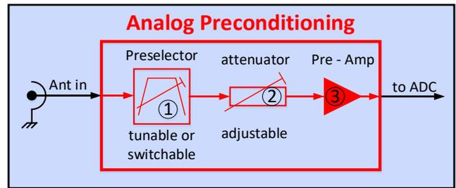
Δ Fig. 2 Analogue preconditioning for direct sampling
