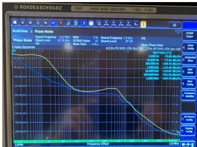
Δ Fig. 13 Phase noise of an analogue Transmitter
