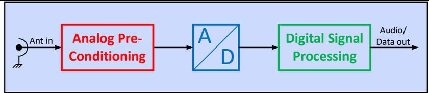
Δ Fig. 1 General and simplified SDR architecture
