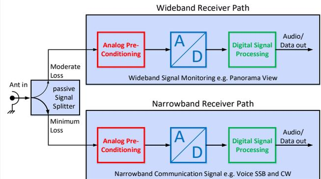
Δ Fig. 5 SDR Receiver Structure
