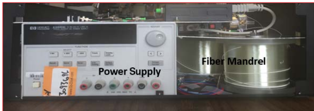
▲ Fig. 6 Front view of the OEO synthesizer, showing the power supply (left), 1 and 5 km fiber mandrels, laser driver and other components.
