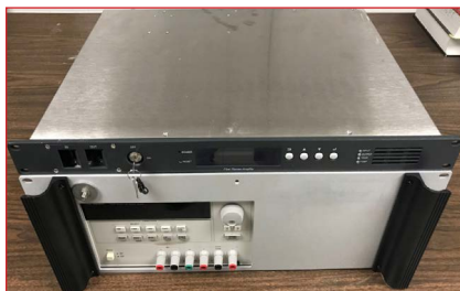
▲ Fig. 7 Complete SILPLL OEO system.
